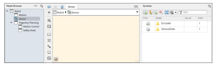
**3** Select the **SensorData** output and view the interface in the **Property Inspector**. You can access this interface like a Simulink bus signal.
